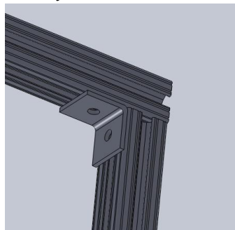
Figure 14. The 90 degree angle brackets used to connect the legs and base.
