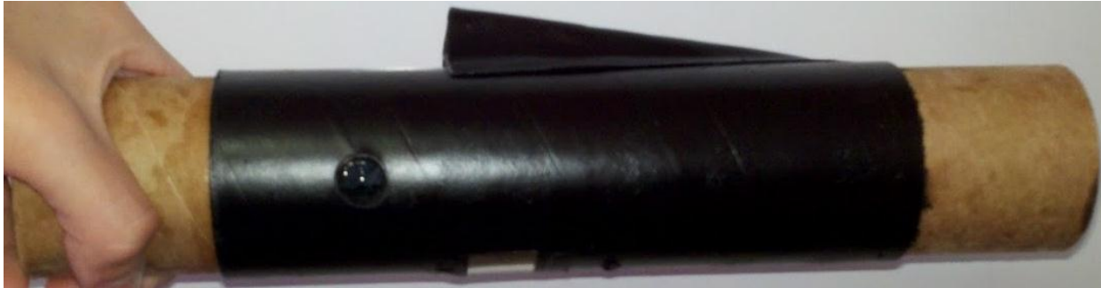
Figure 8. Exterior of avionics bay with periscope (top), window (bottom) and access holes.
