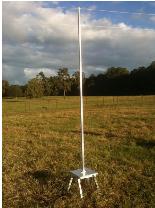
Figure 3. Launch pad set-up prior to having the rocket mounted.
