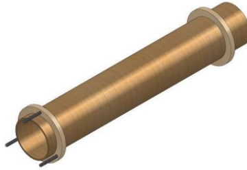
Figure 17. Mounting of the centering rings onto the 38 mm tube using epoxy
