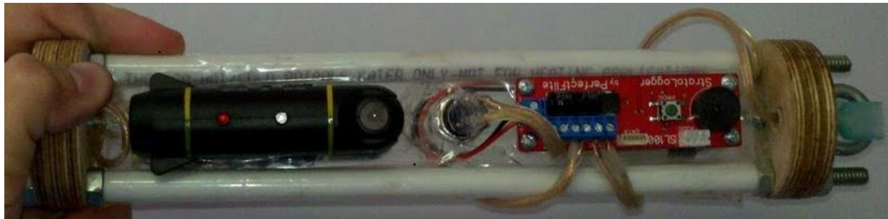
Figure 6. Top view of avionics bay showing ground-view camera and altimeter.
